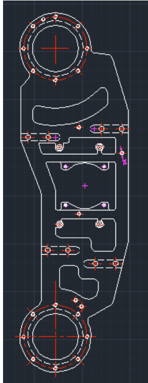
HUBO upper- inside leg AutoCAD drawing
